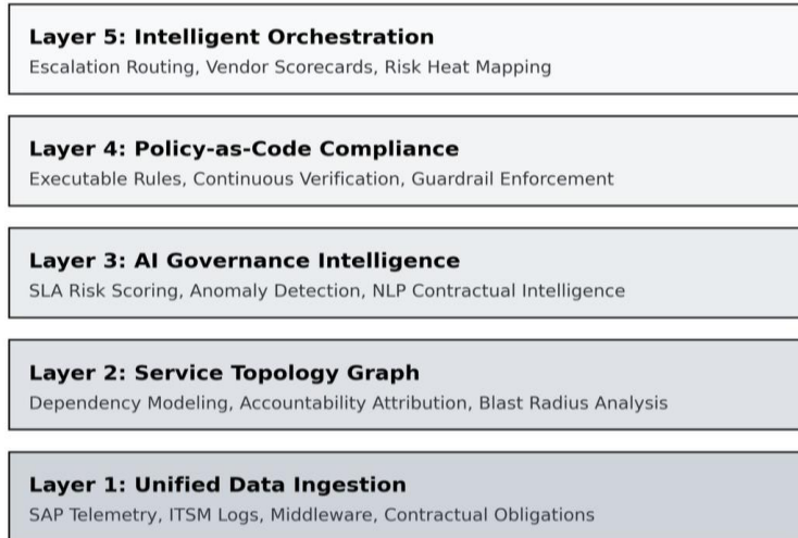
Fig 2: Five-Layer Architecture of the AI-Driven Governance Control Plane
