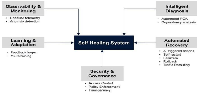
Fig 2: AI-Driven Self-Healing System Architecture for Autonomous Reliability and Security Management
